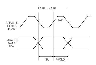
Fig. 4 Input Clock / Data Timing
