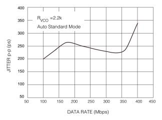
Fig. 5 Output Jitter
