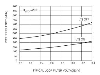
Fig. 7 VCO Frequency vs Loop Filter Voltage
