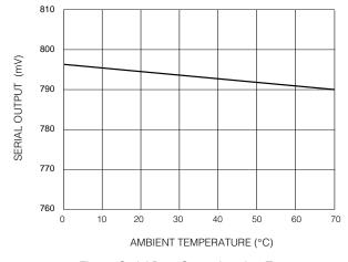
Fig. 6 Serial Data Output Level vs Temperature
