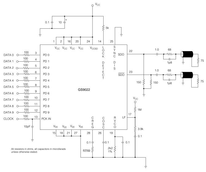
Fig. 9 GS9022 Application Circuit
