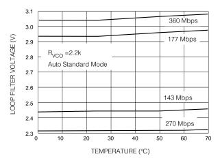
Fig. 8 Loop Filter Voltage vs Temperature
